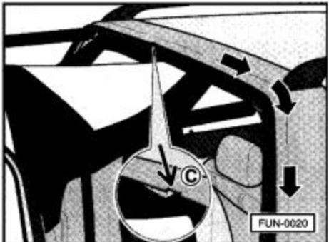
Take the roof cover out of the packaging. Guide the right side of the cover from the middle - see arrow C - into the guide in the frame of the driver's cab and pull it to the right (in the direction of the arrow) to the end of the guide.
