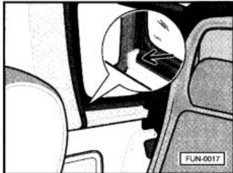
If necessary, tension the cover equally by pushing the tensioning element forwards. Fasten the loose side parts of the cover to the tensioning element using Velcro. Pull the tabs inwards at the front and also attach them to the frame of the driver's cab using Velcro fasteners - see arrow.
